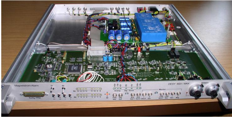
Figure 3.2: The Fast Magnet Current Change Monitor
